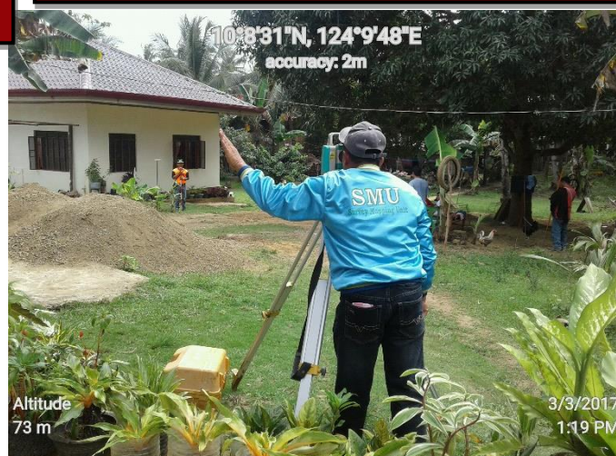
Using the Prism Pole to shot the corners of boundary located at Taytay, Getafe, Bohol last March 3, 2017
