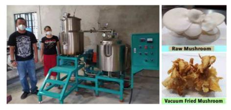
Green Thumb Farm in Sambog, Corella, Bohol, a beneficiary of the Small Enterprise Technology Upgrading Program (SETUP) of DOST, acquired and installed one (1) unit Vacuum Fryer to produce mushroom chips and other mushroom-based products.
