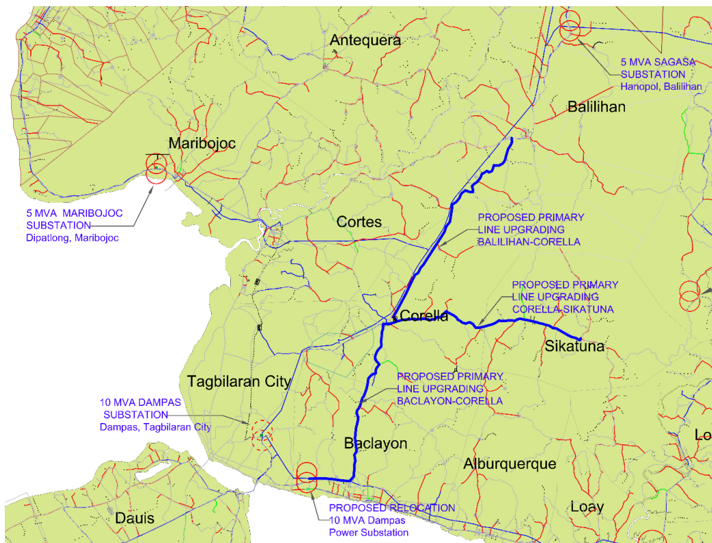
Figure 6-4 13.2-kV Primary Distribution Line Upgrading (Balilihan—Corella)
