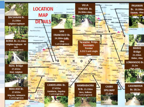
PROPOSED LENGTH CONFIGURATION OF TEMPORARY/EMERGENCY Single Lane Modular Steel Bridges in Bohol Province
