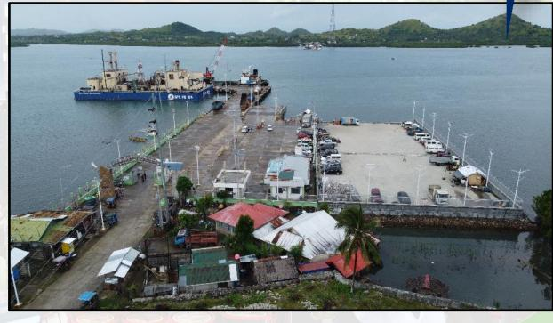
There are shallow areas within the channel and maneuvering areas. This project is needed to be able to have a safe berth for foreign and cruise ships. Proposed Design Depth = -10.00m. (Port of Catagbacan, Loon) **ESTIMATED VOLUME: 108,000.00 CU.M**
